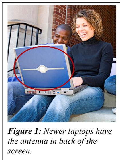
**Figure 1:** Newer laptops have the antenna in back of the screen.
